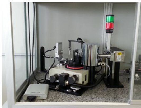
Figure 2.2: Bruker Diffractometer Model D8 Focus employed for XRD measurements.
