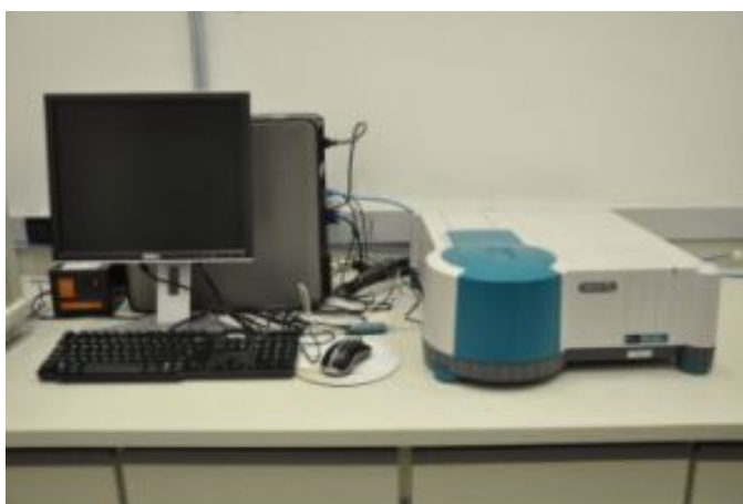
Figure 2.6: UV-VIS Spectrophotometer Cary 50-Varian.
