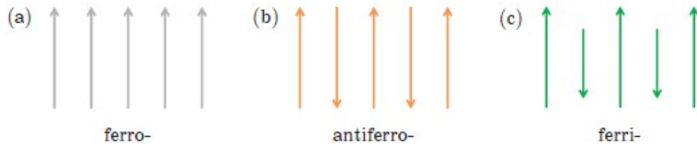
Figure 1.9: Schematic showing spontaneous ordering of magnetic moments in (a) ferro-, (b) antiferro- and (c) ferri-magnets.
