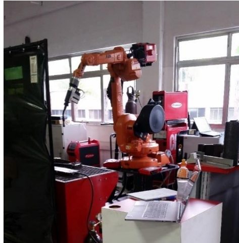
Figure 18: ABB robot with a CMT (Cold Metal Transfer) Fronius® power supply.
