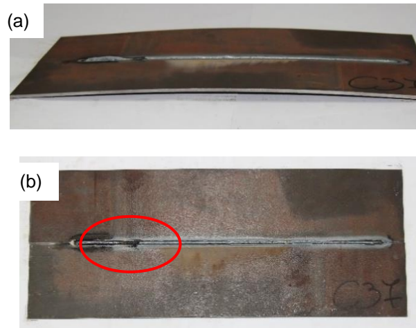
Figure 20: Welding defects on the AHSS900 base metal welded by pulsed transfer, distortion(a) and excess penetration (b).
