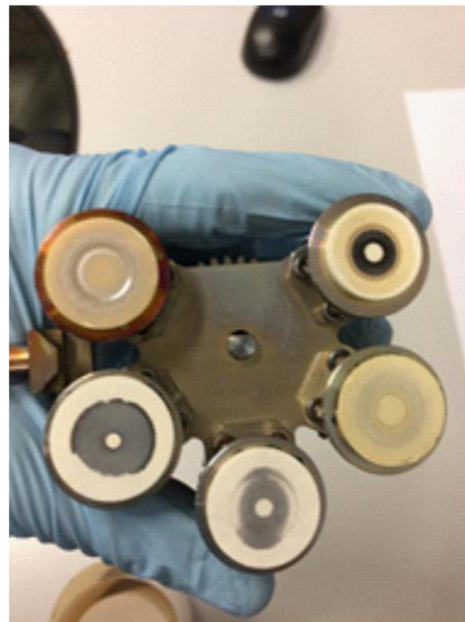
Figure 6: a) Pulsed Laser Deposition System, b) tantalum oxide based and mixed zirconia and tantalum oxide targets
